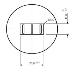
The gauge shall be made of hard corrosion-resistant metal (e.g., stainless steel). The total mass of the gauge shall be 80N (8.15kg).
