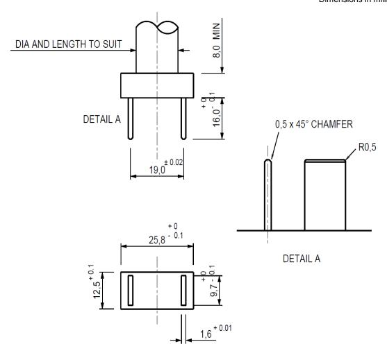
The test is made with the engagement face of the socket-outlet horizontal and the shutters (if any) open. The gauge is applied under its own weight in every possible position.
