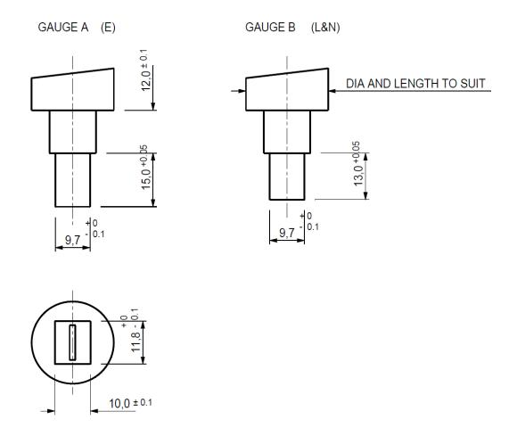
The gauge shall be made of hard corrosion-resistant metal (e.g., stainless steel. The total mass of the gauge shall be 3N (306g).
