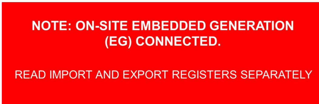
Figure 8 — Example of labelling for metering points (Colouring and other requirements to be confirmed with the utility).
